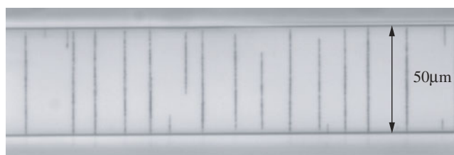
Figure 1. Chains of particles aligned with the magnetic field in a square capillary tube of 50\ \mu\text{m} (optical microscopy, \times 100 objective).
